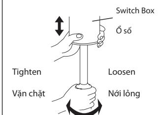
To adjust height. Loosen the Free Stop Cap. Adjust the fan height by moving the switch box to desired height and retighten the Free Stop Cap.
